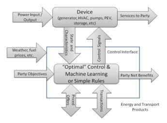
**Figure 4 : End Device Transactive Operations**
